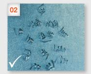
Loosely rolled chips - correct cutting data
